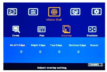
User can use [Overlap] function to changes the cropping area, aspect ratio and image position. It can also execute Bezel compensation and correct misalignment in video wall installation.
