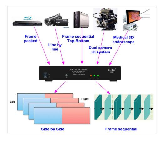
User can apply dual camera FHD 3D signal to G901. G901 can be set at POP mode and output 4k/2k side by side image for 3D display.
