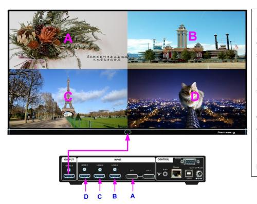
For 4 input sources, at least one input should come from DP port. If the signal source is only in HDMI format, user can use HDMI to DP converter to convert HDMI to DP. Please note that this kind of converter requires external power source. It is different from DP to HDMI adapter without power supply.
