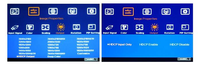
Three sub-menu under [Image Properties]  $\rightarrow$  [Output]  $\rightarrow$  [HDCP Output] settings:
