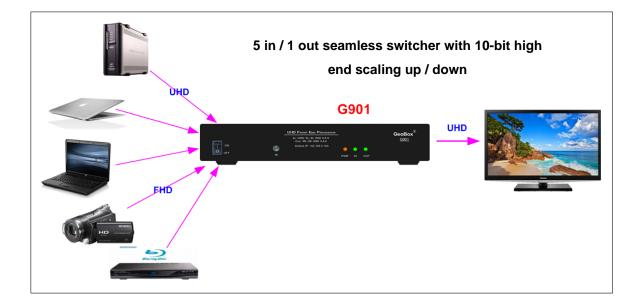
All HDMI input sources can support up to 4k/2k/60Hz 4:4:4 input resolution. DisplayPort input can support up to 1080MHz (7680\*4320/30Hz). The output resolution can be from 1024\*720 to 4096\*2160/60Hz.
